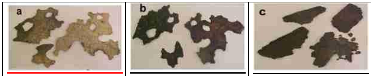
FIGURE 4. Specimens after testing in different environments without (a) and with inhibitors (b)
