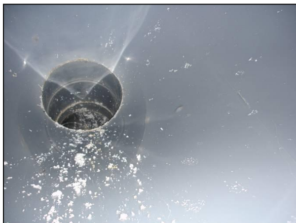
Figure 9 - Inside view of the ECTFE liner after 7.5 years of service (bottom)
