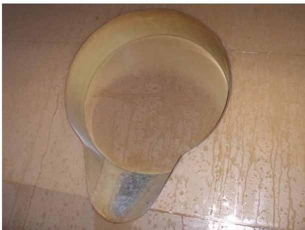
Figure 5 – ECTFE liner after 10 years of service
