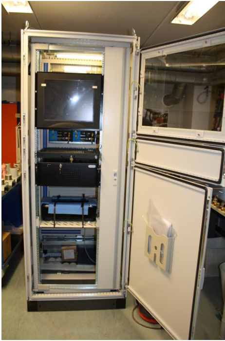
Figure 1: Cabinet for an integrated monitoring solution for an offshore platform, covering corrosion probes, acoustic sand monitors, field signature measurement for erosion monitoring, and acoustic pig detectors.
