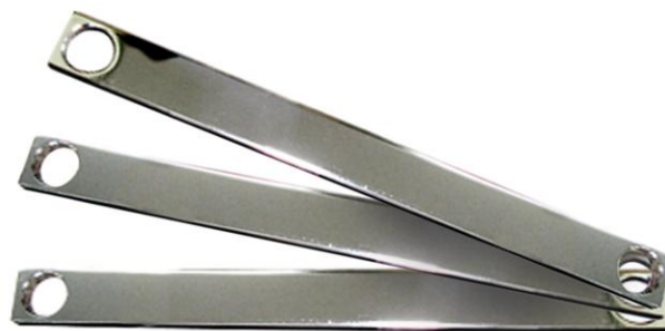
Figure 3. Inconel 600 plates polished up to 1 \mu\text{m} .
