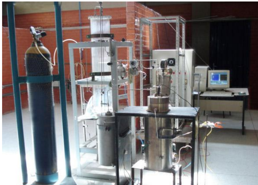
Figure 6. Facility for SCC tests.
