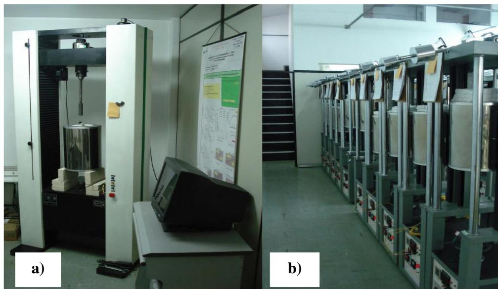
**Figure 2** – Equipment used in this study: a) universal machine used in hot tensile testing and b) row of 10 machines used in creep testing.
