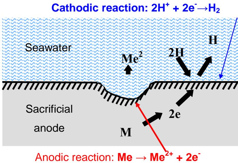
Figure 02 – Schematic representation of the electrochemical reactions involved in the cathodic protection process.
