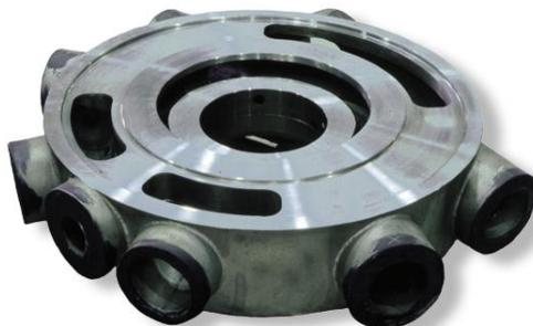
Figure 07 – Steam chest made by the HIP process, in the as-HIPed condition, with a finish machined surface.
