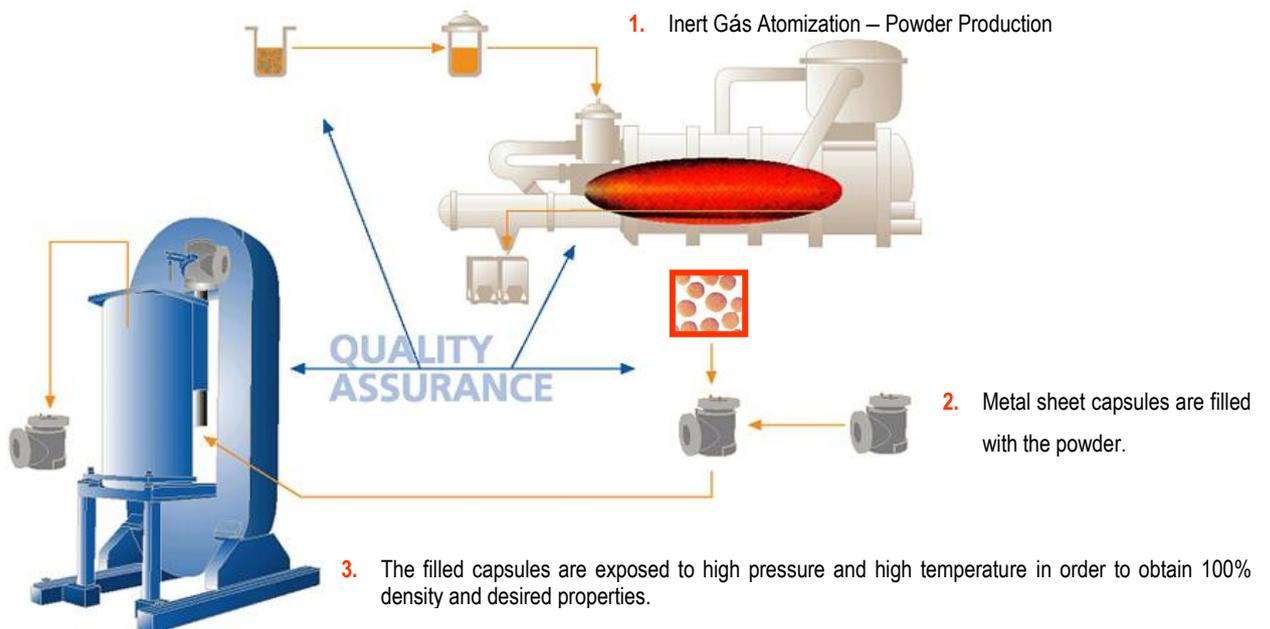
Figure 06 – Scheme of the steps of the HIP process performed by Sandvik Powdermet.
