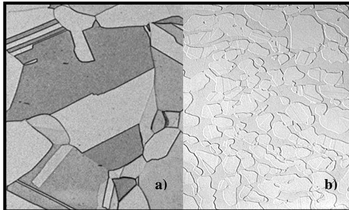
Figure 05– Typical Microstructures for Austenitic (a), and Duplex material (b).
