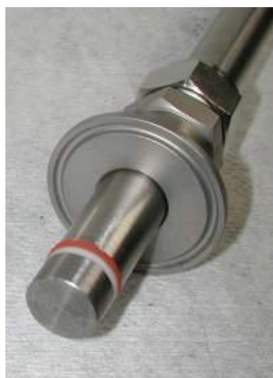
Figure 8: Localized corrosion probe used for flow loop testing
