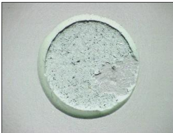
FIGURE 9: Coating C – TSA plus epoxy novolac with glass flakes. Pull-Off test, after fatigue resistance test – cohesive failure.
