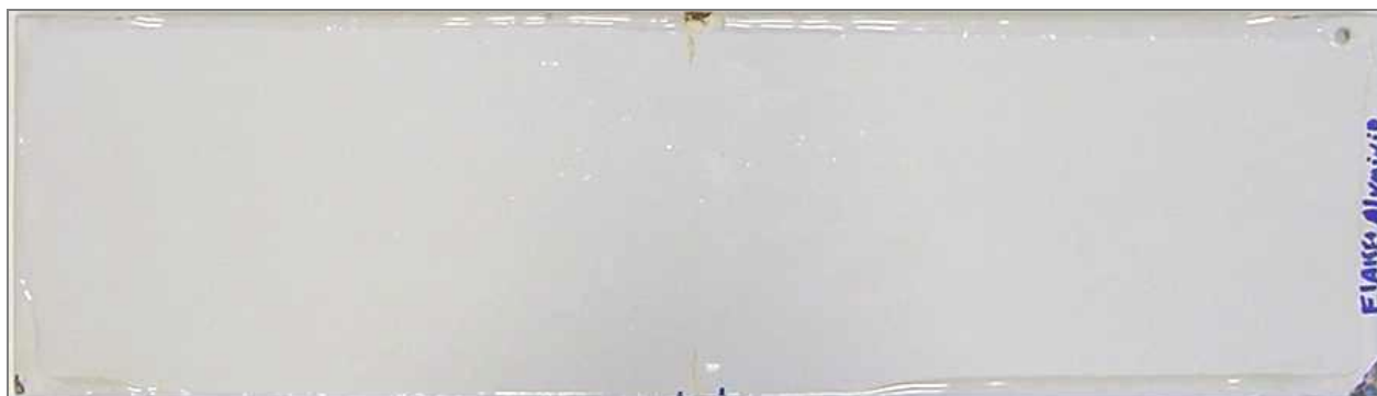
FIGURE 10: Coating C – TSA plus epoxy novolac with glass flakes, after fatigue resistance test. There was no cracking in the coating.
