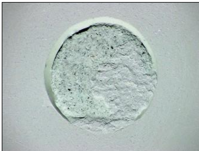
FIGURE 7 – Coating B – Epoxy novolac with glass flakes. Pull-Off test, after fatigue resistance test – cohesive failure.
