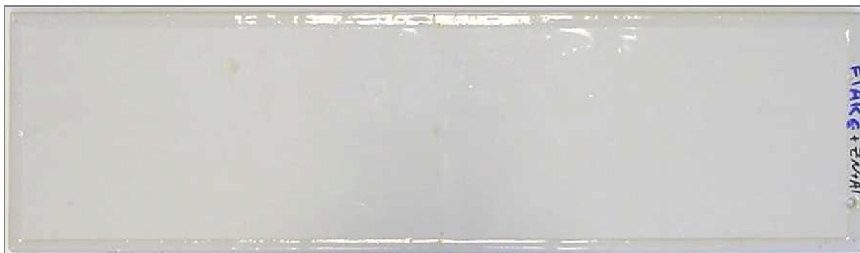
FIGURE 12: Coating D – TSZA plus epoxy novolac with glass flakes, after the fatigue resistance test. There was no cracking in the coating.
