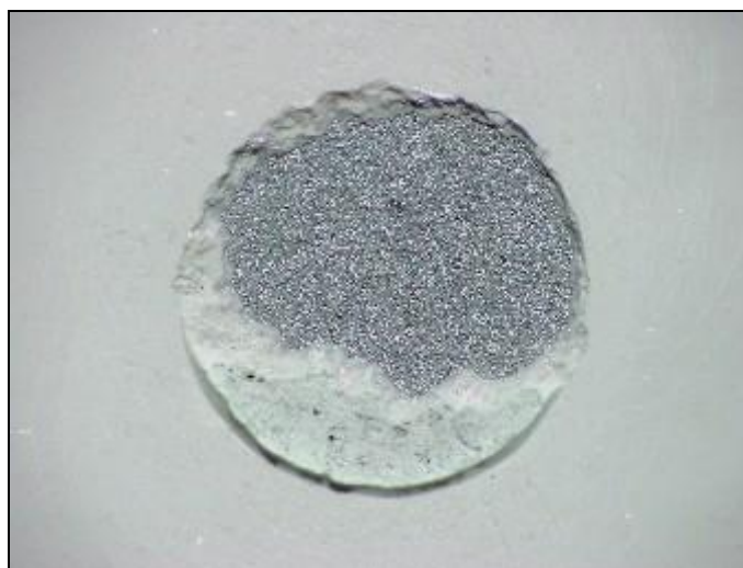
FIGURE 11 – Coating D - TSZA plus epoxy novolac with glass flakes. Pull Off test, after fatigue resistance test – adhesive failure.
