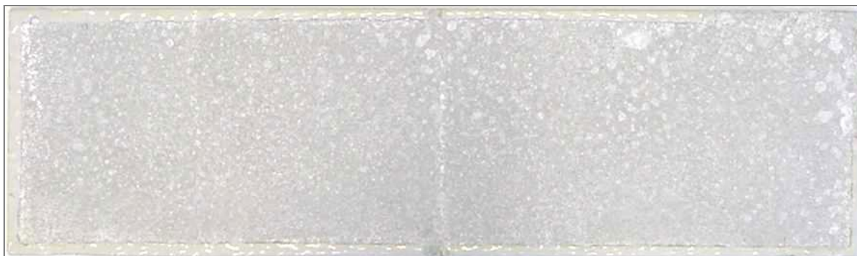
FIGURE 6 - Coating A - TSA sealed with epoxy after the fatigue resistance test. White corrosion products were observed.
