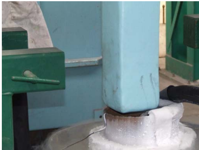
Figure 2a – Test specimen ready to be immersed in LN 2 as part of the “South Hook” test
