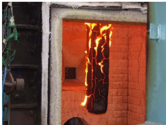
Figure 2c – Test specimen after 60 minute UL1709 fire test as part of the “South Hook” test
