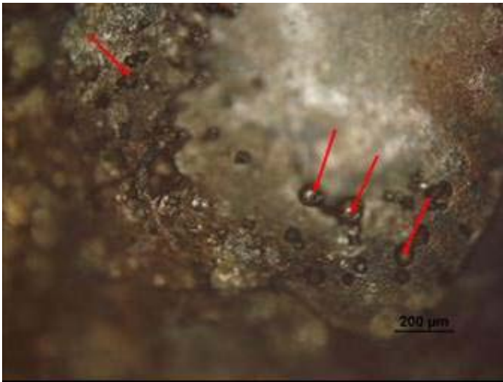
Figure 6 - Photograph of the filter. The attacked zone by pitting is indicated (10 X)
