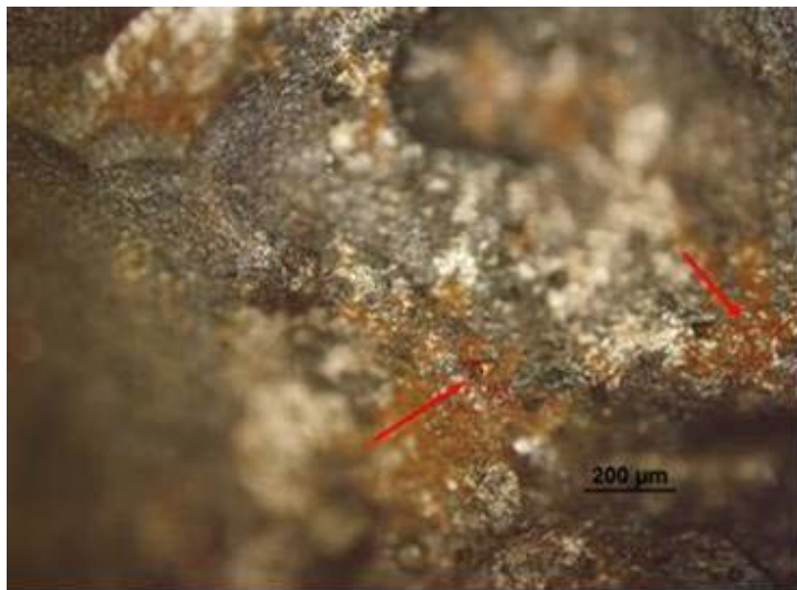
Figure 5 - Photograph of the filter. Orange colored zones (indicated) and brilliant streaks can be observed (10X)
