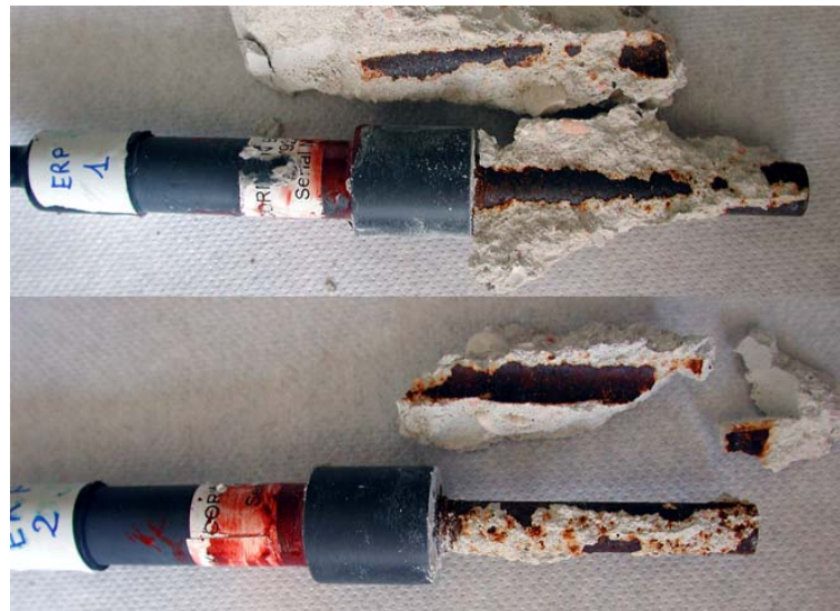
Fig. 7 - ERP1CO 2 probe (up) and ERP2CO 2 probe (down) pulled out from CO 2 1 specimen at the end of the experimentation.
