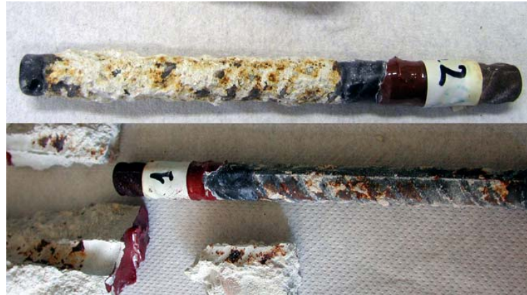
Fig. 6 - Rebars pulled out from specimen CO 2 1 at the end of the experimentation.
