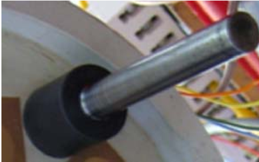
Fig. 2 - ERP probe before embedding it in concrete specimen.
