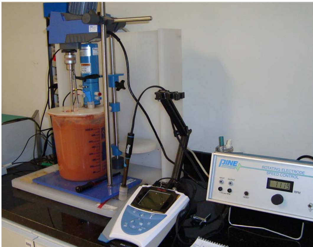
Figure 2 – Schematic diagram of the proposed apparatus to evaluate the corrosion-erosion process in bauxite sludge. (1) 5000 cm 3 polypropylene vessel; (2) stirrer just to maintain the homogeneity of the sludge; (3) rotating cylinder working electrode; (4) reference electrode; (5) stainless steel auxiliary electrode; (6) and (7) vents; and (8) electric motor.
