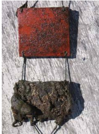
Photograph No. 1: General aspect of the panels with AMERCOAT 235 + ABC # 3 covering (upper panel). Control panel (lower panel). 365 days of immersion.
