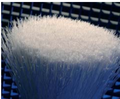
Photo 7 - Hollow Fiber Membranes Made from PVDF for Water Purification
