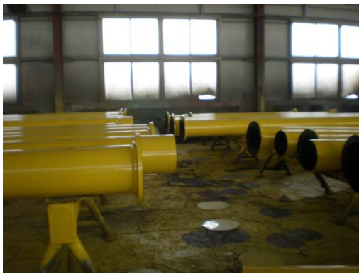
Figure.3: Example showing that blasting and painting of piping at workshop was of good quality. However paint work experienced a lot of mechanical damage, during transport and installation in addition to dirt on site.
