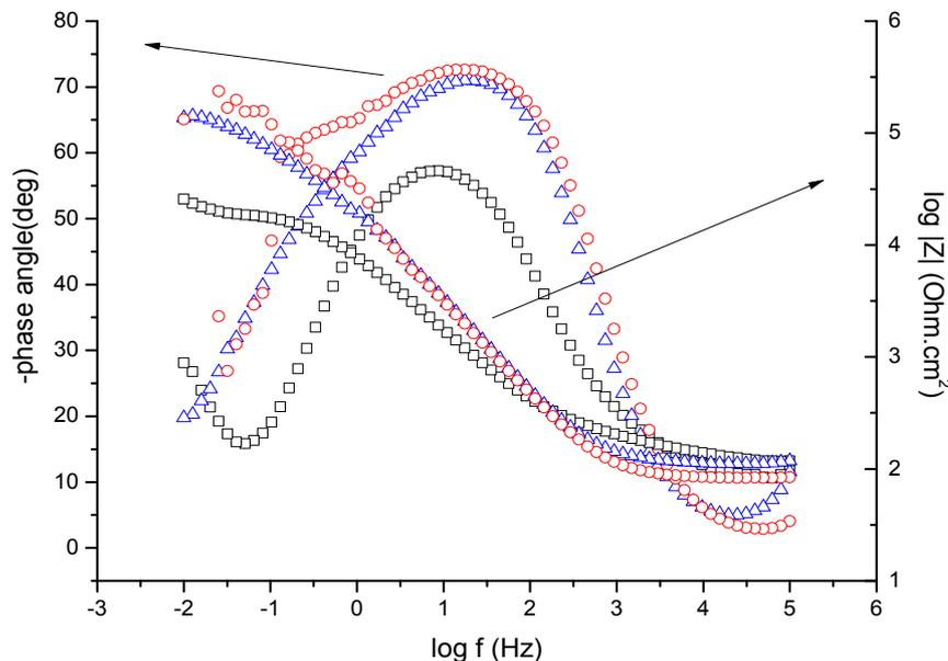
**Figure 6 - Bode plots for aluminum immersed along 72 h in  $4.0 \text{ g.L}^{-1}$  ( $\Delta$ ) and  $6.0 \text{ g.L}^{-1}$  ( $\circ$ ) of tannin and in absence of tannin ( $\square$ ).**
