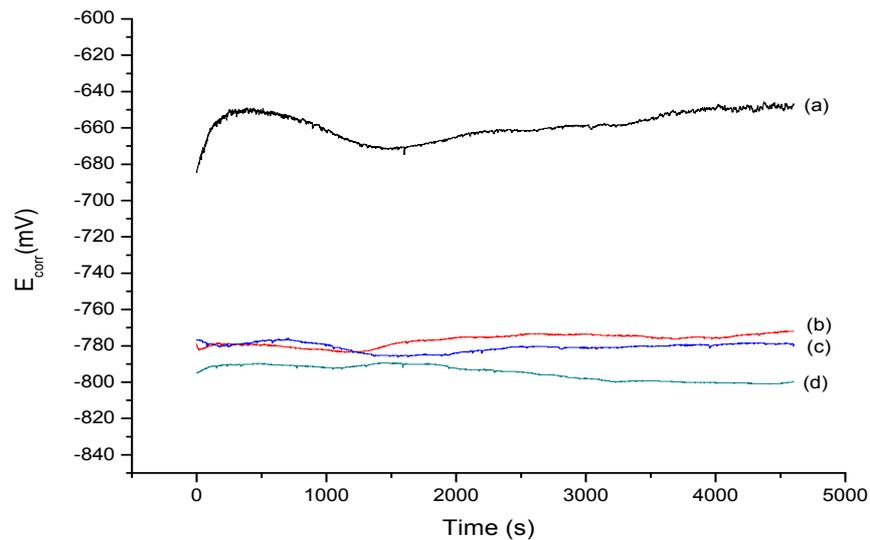
**Figure 1 - Corrosion potential ( $E_{\text{corr}}$ ) concerning the reference electrode (SCE) curves of aluminum immersed along the time in presence of tannin -  $4.0 \text{ g.L}^{-1}$  (b),  $5.0 \text{ g.L}^{-1}$  (c) and  $6.0 \text{ g.L}^{-1}$  (d) - and in absence of tannin (a).**
