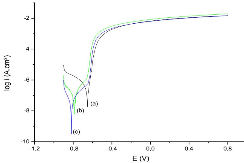
**Figure 4 - Potentiodynamic polarization curves of aluminum immersed along 1 h in the following concentrations of tannin solution: 6.0 gL<sup>-1</sup> (c); 5.0 gL<sup>-1</sup> (b), and the blank sample (a).**
