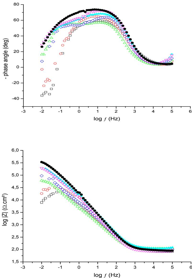
Figure 3 - Bode plots for aluminum immersed along 1 h in the following concentrations of tannin solution:  $6.0 \text{ g.L}^{-1}$  (●);  $5.0 \text{ g.L}^{-1}$  (▽);  $4.0 \text{ g.L}^{-1}$  (☆);  $3.0 \text{ g.L}^{-1}$  (◇);  $2.0 \text{ g.L}^{-1}$  (△);  $0.5 \text{ g.L}^{-1}$  (○) and the blank sample (□).
