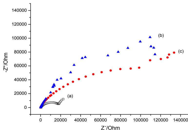
**Figure 5 - Nyquist plots for aluminum immersed along 72 h in 4.0 g.L<sup>-1</sup> (b) and 6.0 g.L<sup>-1</sup> (c) of tannin and in absence of tannin (a).**
