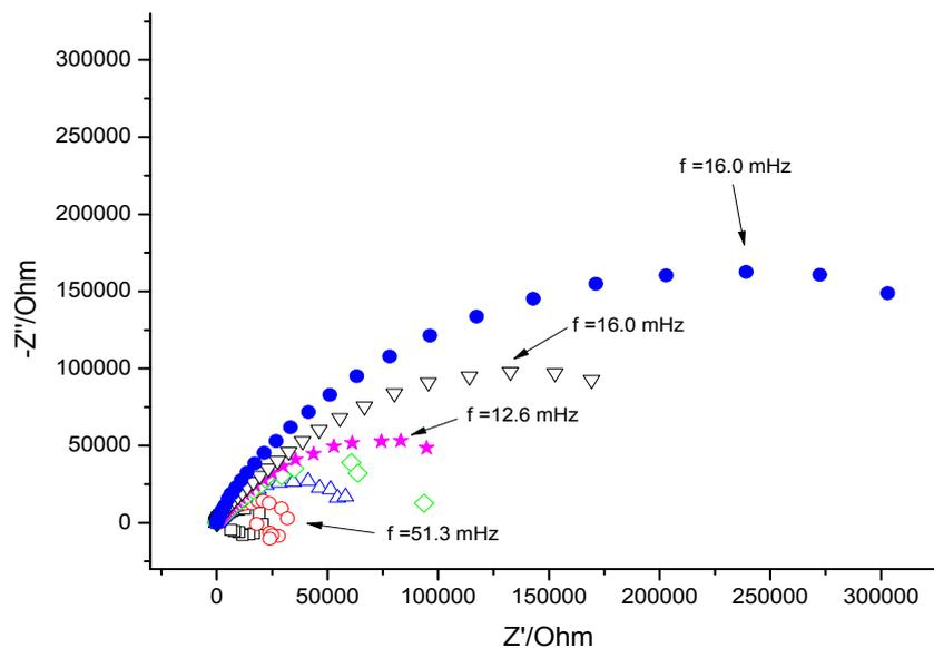
**Figure 2 - Nyquist plots for aluminum immersed along 1 h in the following concentrations of tannin:  $6.0 \text{ g.L}^{-1}$  (●);  $5.0 \text{ g.L}^{-1}$  (∇);  $4.0 \text{ g.L}^{-1}$  (★);  $3.0 \text{ g.L}^{-1}$  (◇);  $2.0 \text{ g.L}^{-1}$  (△);  $0.5 \text{ g.L}^{-1}$  (○) and the blank sample (□).**
