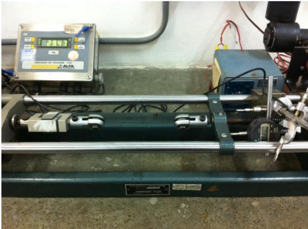
**Figure 1 - Horizontal tensile used for the mechanical tests, working length wire of 130mm.**
