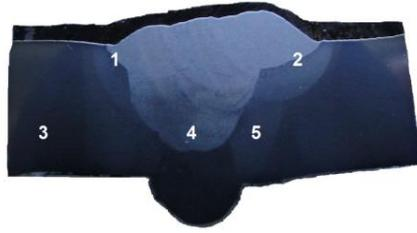
**Figure 1 - Photo of the weld zone of the API X52 carbon steel, with the positions that images were taken.**
