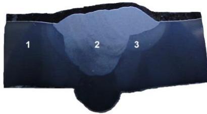
**Figure 13 - Photo of the weld metal API X52 carbon steel, with the positions of the captured images.**
