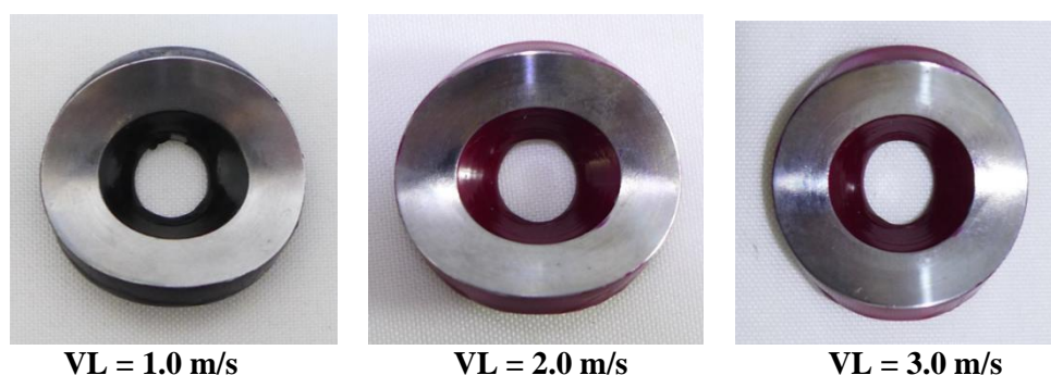
Figure 11. Surface Photos of Weight-Loss Coupons After Inhibitor U Test (Before Cleaning), Flow Loop Test Results, 30 mg/L
