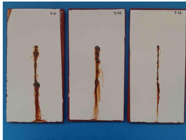
Figure 10 Aspect of the panels I-21, I-22 and I-23 after exposure to neutral salt spray.
