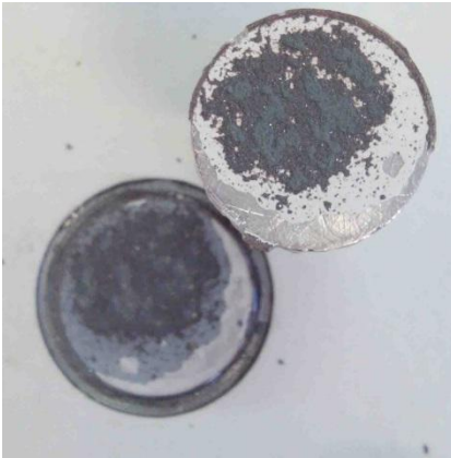
Figure 11 Aspect of the dolly (upper side) and surface (lower side) of performing pull-off test characteristics after Salt Spray exposure
