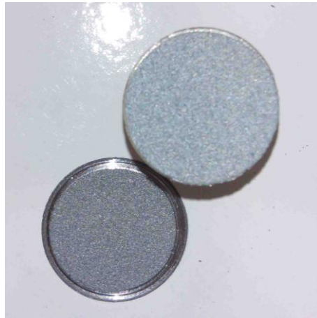
Figure 8 Aspect of the dolly (upper side) and surface (lower side) of pull-off test characteristics
