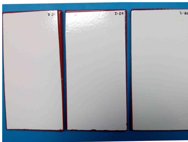
Figure 16 Aspect of the panels I-28, I-29 and I-30 after exposure to humidity in condensation-water atmosphere.
