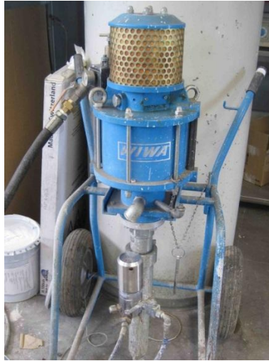
Figure 3 High pressure pump Airless Professional Series from WIWA Wilhelm Wagner GmbH & Co. KG
