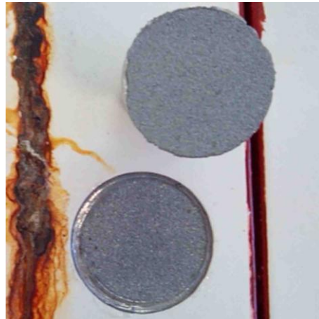
Figure 13 Aspect of the dolly (upper side) and surface (lower side) of performing pull-off test characteristics after Salt Spray exposure
