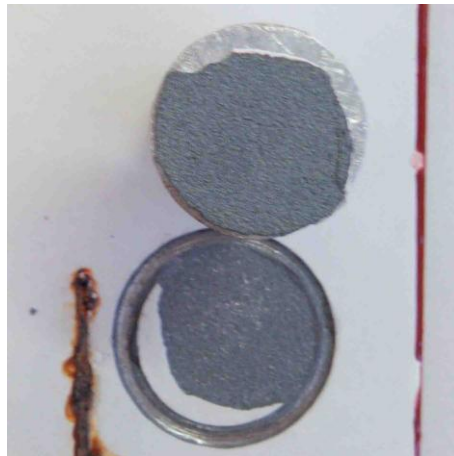
Figure 15 Aspect of the dolly (upper side) and surface (lower side) of performing pull-off test characteristics after Salt Spray exposure
