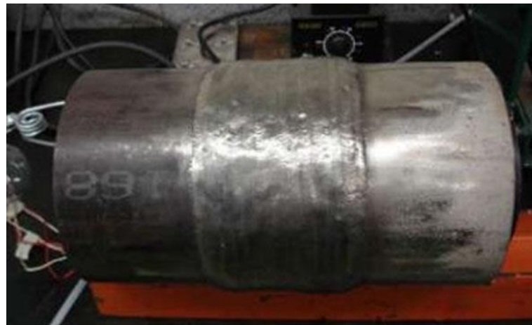
Figure 2 – Weld overlay applied at welded region dissimilar joint.
