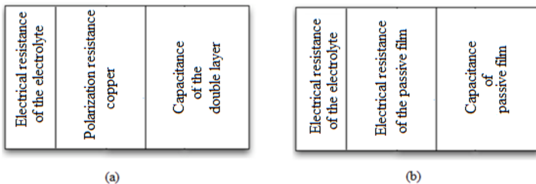
Figure 1 Block diagram of the electrical parameters for the electrochemical system proposed: (a) copper electrode polished state and (b) copper electrode on passivation film
